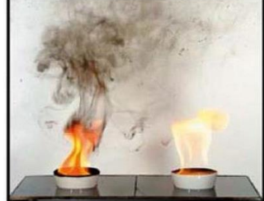
Burning of conventional diesel (left) and paraffinic diesel (right). Ref. ASFE
