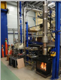
INERIS dilution system for Wood stove / Fireplaces
