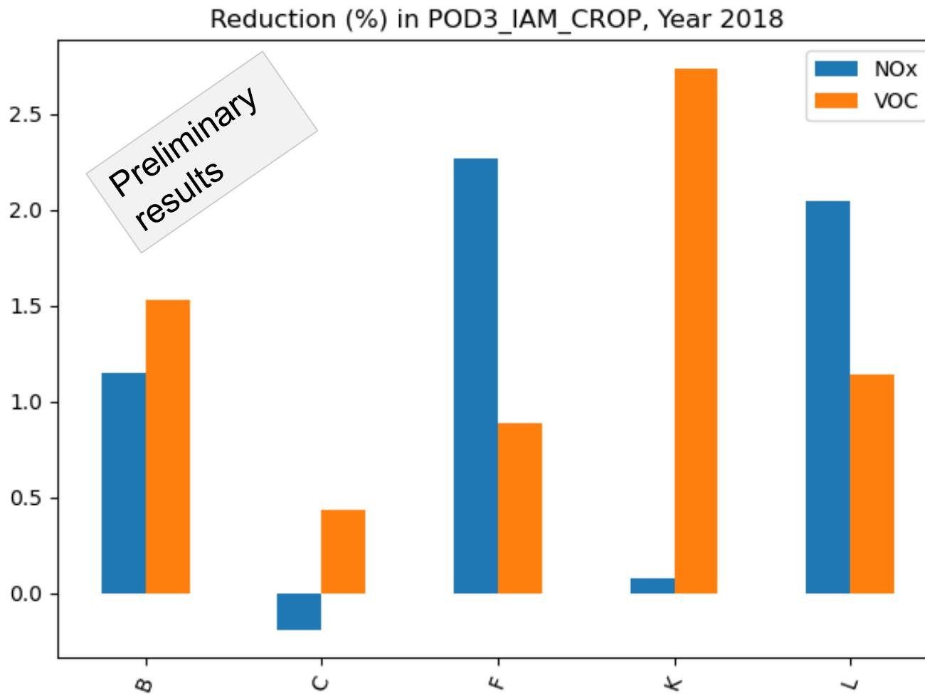
Reductions in mean of POD3-IAM-CROP over central Europe in 2018 due to removal of NO<sub>x</sub> or VOC emissions in GNFR classes B (Industry), C (small combustion), F (road transport), K (Agriculture livestock) and L (other agriculture)
