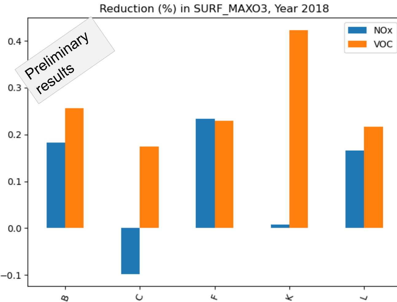
Reductions in mean of daily max. O<sub>3</sub> over central Europe in 2018 due to removal of NO<sub>x</sub> or VOC emissions in GNFR classes B (Industry), C (small combustion), F (road transport), K (Agriculture livestock) and L (other agriculture)
