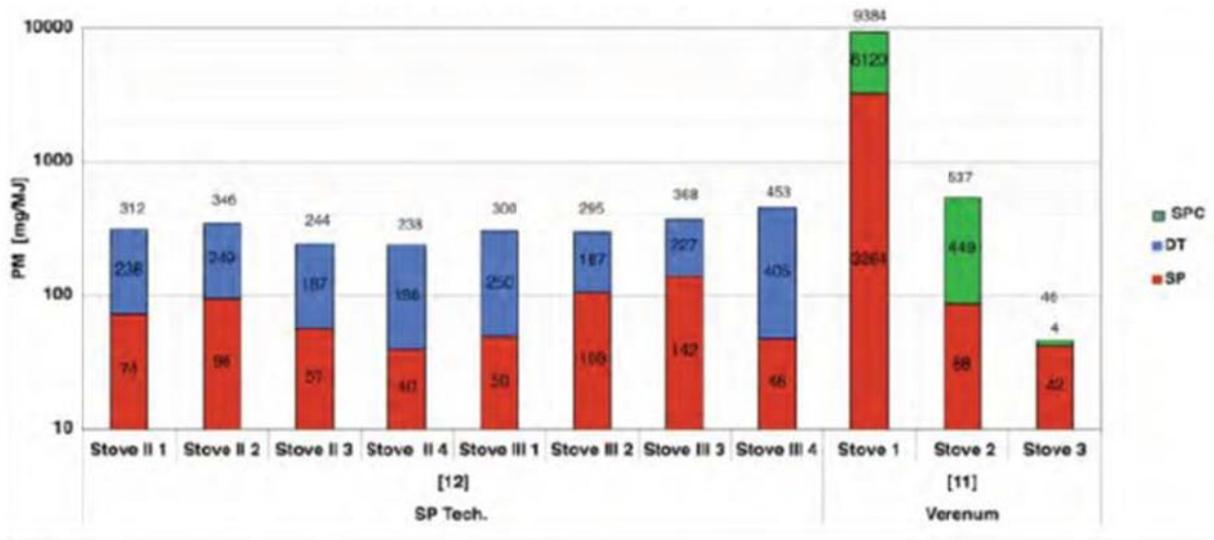
Figure 2: Comparison of PM emission factors on solid particles (SP), particles in dilution tunnel (DT), and solid particles plus condensables from impinger (SPC) for wood stoves.
